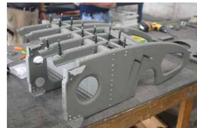
Above, top to bottom: A good portion of the interior structure of the wings was either reusable or used to make patterns to create new parts.
