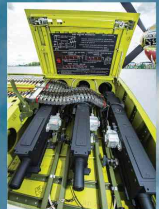
Six replica Browning .50-cal machine guns were installed in Was That Too Fast .
