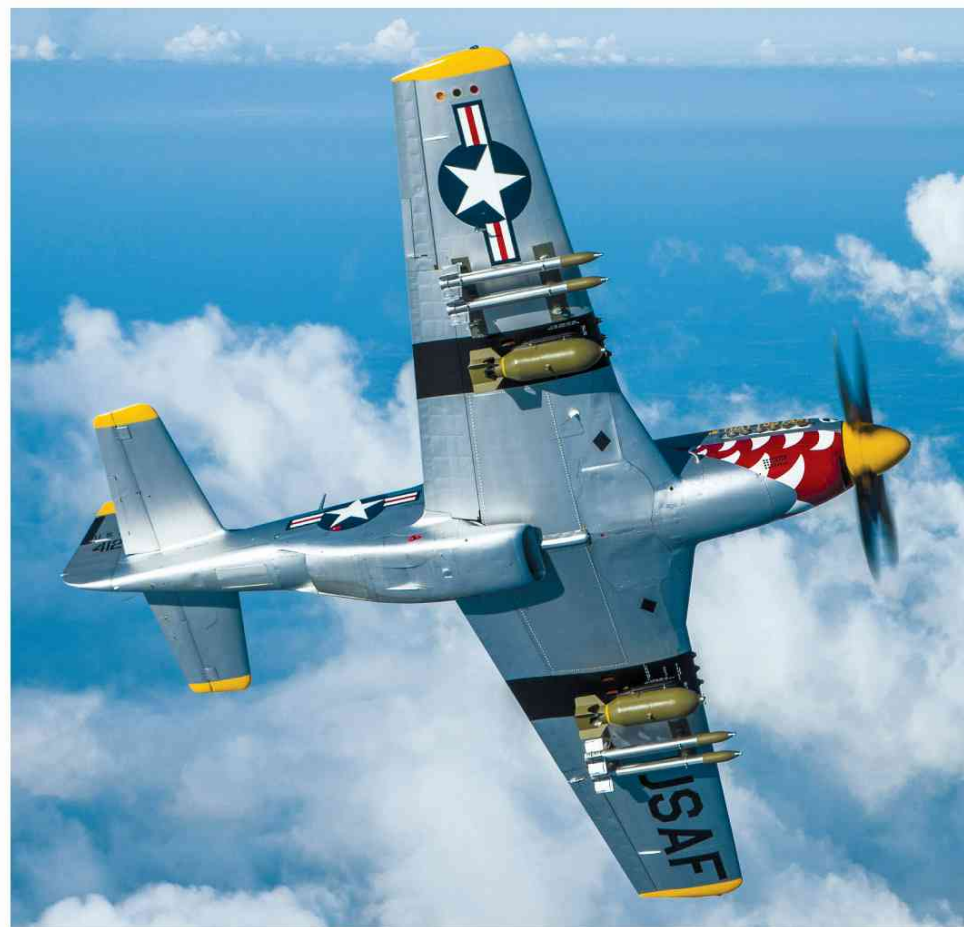
Finding a new old stock rocket stub field installation kit was essential to completing the aircraft's Korean War configuration.
